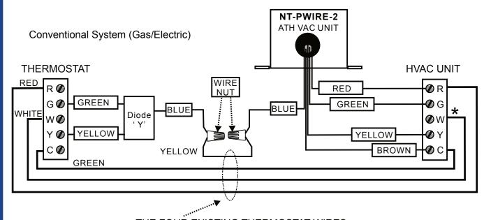
THE FOUR EXISTING THERMOSTAT WIRES
