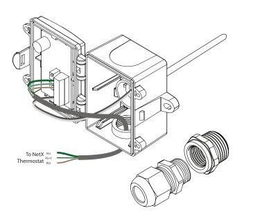
NOTE: A 1/2" NPT threaded connection hole is provided at the bottom of the enclosure. If installing in an environment that needs to be water tight, screw the EMT or cable gland connector (not included) in until tight. It is recommended that weatherproof EMT or cable gland fittings be used.
