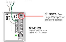
2. Connect wires to each additional sensor in the following manner.
