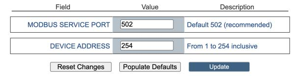
Here you can configure the device's MODBUS SERVICE PORT and DEVICE ADDRESS. The recommended value for the MODBUS SERVICE PORT is 502. Care must be taken to prevent conflict between other ports used on the thermostat and the network. As such is it recommended NOT to use ports 0, 80, 443, and 10001 as these ports are used for other communication.
