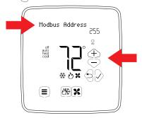
**NOTE:** The Modbus address may also be set over Modbus communications
