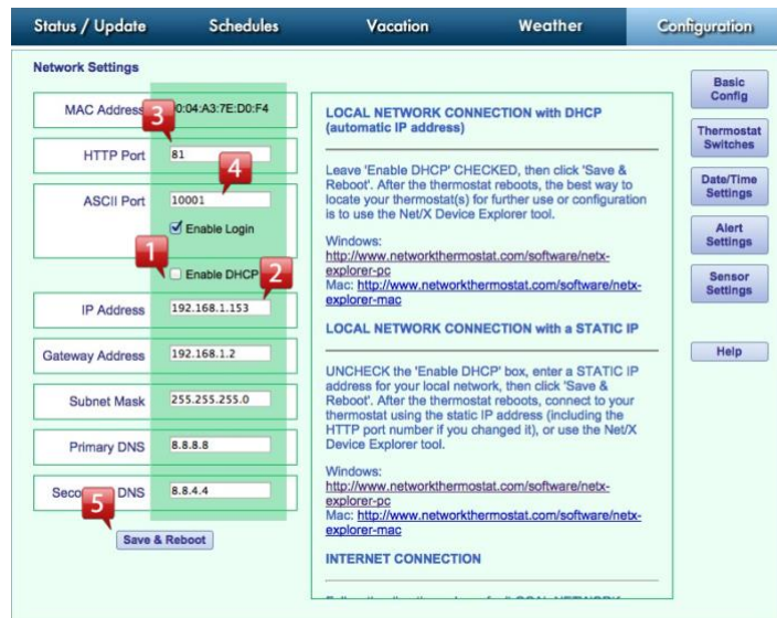
Figure 8 - Static IP Address, HTTP Port 81, ASCII Port 10001
